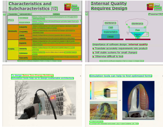
Figure 7. Refined bounding boxes from text detection. The results are automatically verified in order to remove false alarms.
