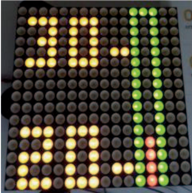
Fig. 8. Task 4 – Draw the measured and calculated temperature value in a given thermometer template on the LED display
