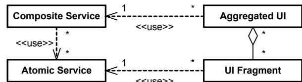
Figure 7: UML diagram showing the artifacts of service composition and user interface aggregation.
