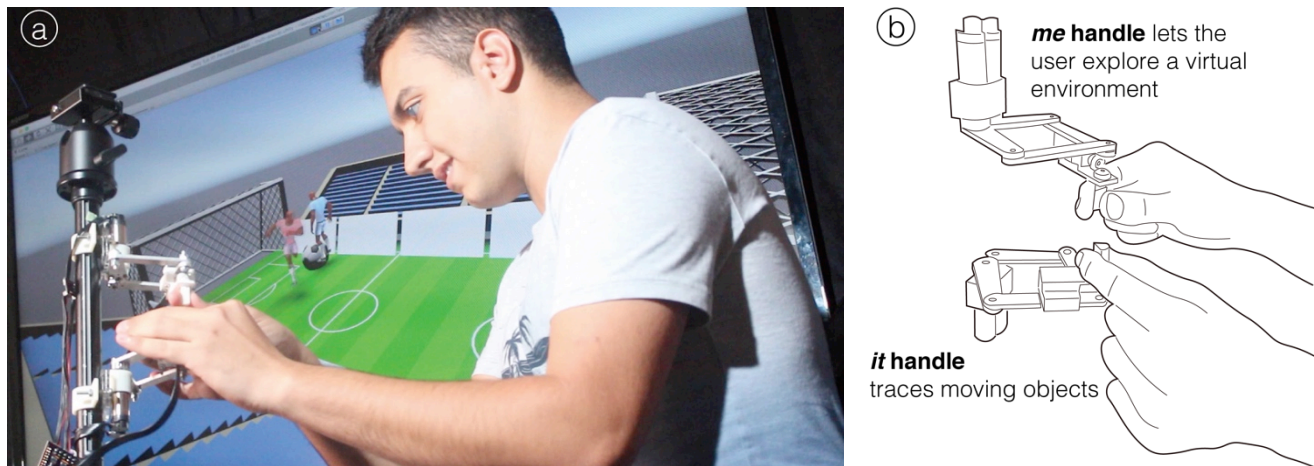
Figure 1: (a) This blind user is playing a real-time soccer game. (b) The DualPanto bimanual haptic device enables this. The user moves the me handle to move their avatar around the virtual world. Force feedback allows users to feel virtual walls, such as the edge of the field, and prevents users from pushing through them. The it handle moves by itself, enabling users to feel where the ball or opponent is located. Users aim by turning the haptic knob on the me handle ; a foot pedal shoots the ball.
