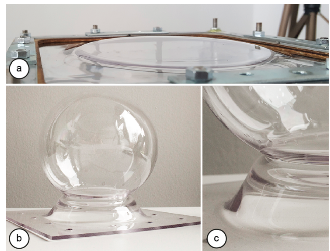
Figure 20: First steps of making a head sculpture with neck. (a) outline shape for neck, (b,c) adding the head.
