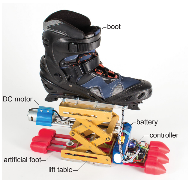
Figure 2: The Level-Up device
