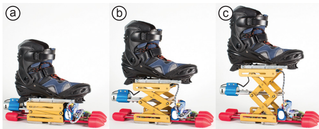
Figure 3: A Level-Up actuating its scissor mechanism
