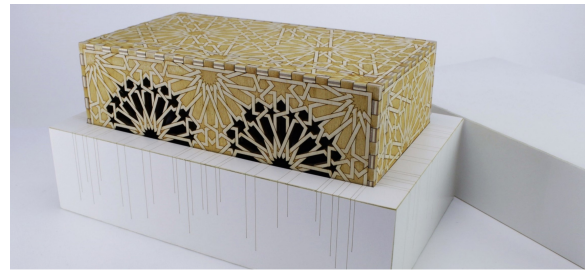
Figure 23: PopCore cuts and engraves from both sides and thus allows engraving decorative designs on this speaker package.
