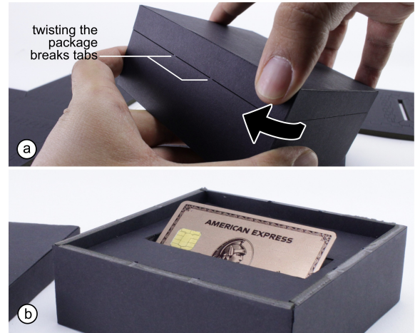
Figure 27: (a) Twisting the top half (b) breaks open the package, leaving an obvious mark that the package has been opened.
