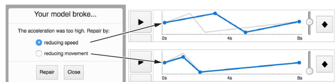
Figure 17: If the user-defined animation breaks the model, TrussFormer offers to automatically reduce the speed or the motion range.
