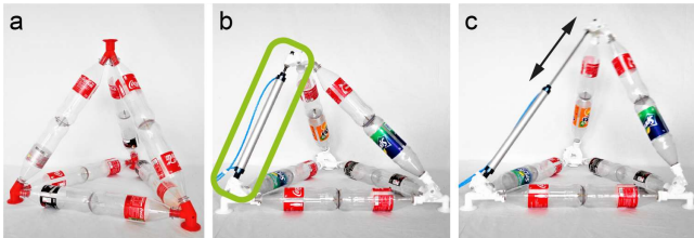
Figure 2: (a) The static tetrahedron (b-c) is converted into a deformable structure by swapping one edge with a linear actuator. The only required change is to introduce connectors that enable rotation.
