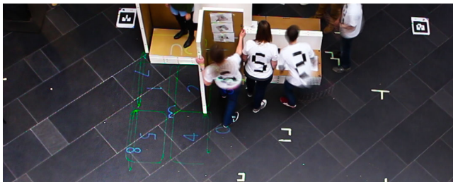
Figure 11: The projected human actuator interface consists of green board outlines and blue human actuator IDs.
