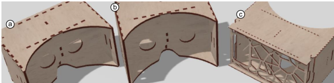
Figure 6: When users have converted the VR headset model to 3D once , the 3D model allows leveraging existing tools (such as kyub [3]) to perform any number of modifications efficiently, such as (a) adjusting the inter-ocular distance, (b) making the headset fit a wider phone by stretching it vertically, (c) or making the headset more comfortable to wear by reducing the weight of the device by decreasing material thickness and removing unnecessary material.
