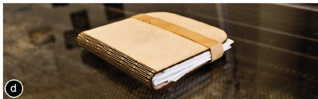
Figure 8: Creating a wooden booklet sleeve by (a) drawing the cover with the polyline tool, then (b) smoothing the corners with the round tool, and (c) making the wood flexible using the bend tool [1].
