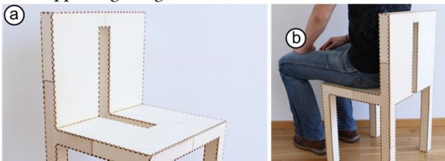
Figure 18: Here a slot cut into the chair reinforces the chair’s seating surface and backrest.
