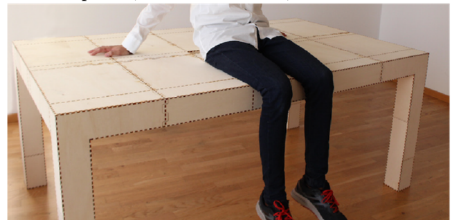
Figure 20: The table from Figure 1 is assembled of separate cells which are capable of holding a human sitting on it.
