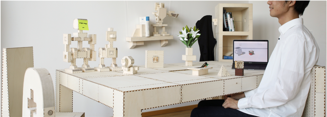
Figure 1: A selection of objects created using kyub , a software system that allows users to design 3D objects for laser cutting. By affording closed box structures, objects made using kyub are very strong. This allows users to make tables, shelves, and chairs that can hold a person. (All shown objects are assembled from 4mm plywood sheets—pressure fit, not glued).
