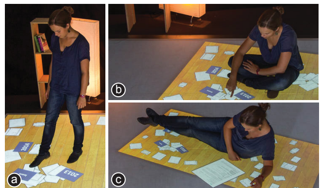
Figure 15: (a) This user is sorting documents for her tax return. Initially, she stands. (b-c) As she sits or lies down, PoseUI positions documents optimally for these poses.
