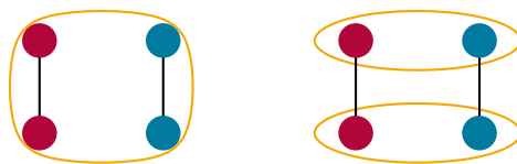
Figure 3.1: Example forest where a cluster of size 4 and two clusters of size 2 incur the same cost. With one cluster of size 4 (left), the inter-cluster cost is 0 and the intra-cluster cost is 4. With two clusters of size 2 (right), both the inter-cluster and intra-cluster cost are 2.
