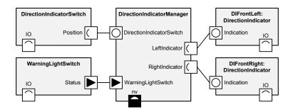
Fig. 4. Design of a car direction indicator system consisting a main managing component and four *Sensor/Actuator Software Components* interconnected through their ports.
