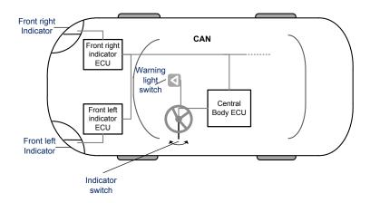
Fig. 1. Hardware components of the simple car direction indicator system example.
