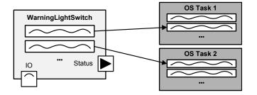
Fig. 5. Exemplary mapping of *Runnables* to *Operating System tasks*.
