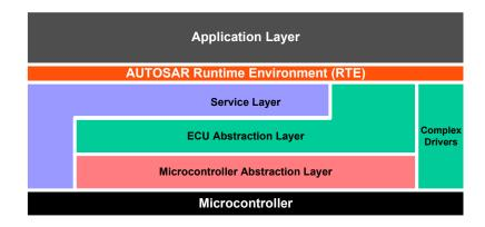
Fig. 2. Layers of the AUTOSAR software architecture
