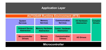
Fig. 3. Stacks of functionality in the *Basic Software layer* of the AUTOSAR software architecture
