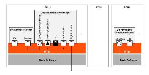
Fig. 6. Communication between AUTOSAR Software Component on the same and on different ECUs, supported by the corresponding Runtime Environment of each ECU.
