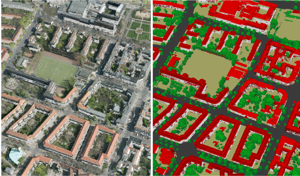
Figure 3: Aerial laser scan of a metropolitan area. Points are colored based on color information extracted from aerial images (left) or based on their respective object classes
