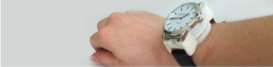
Figure 1: Physical motion displays drag a tacton over the wearer's skin in order to communicate a spatial message. Our self-contained miniaturized prototype is the size of a watch.
