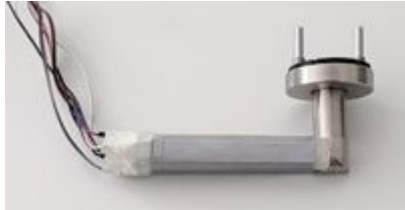
door handle with four touch sensors (top, bottom, front, back)
