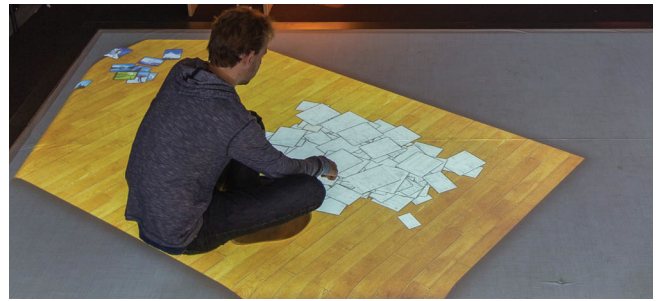
Figure 17: PoseUI transforms the entire floor imagery alongside with the documents, which helps users to understand the current layout information.
