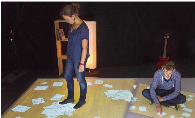
Figure 23: As the user on the right sits down, PoseUI clones the view, allowing each user to work independently.
