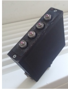
Figure 3: Shear wave transducer consisting of four point contact transducers.
