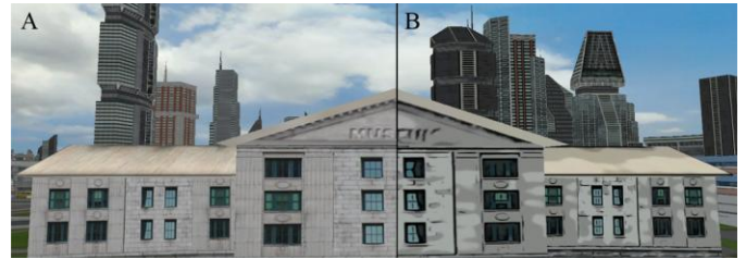
Figure 4. Example of a 3D building using a non-abstracted (A) and an abstracted (B) visualization technique. The abstraction reduces visual complexity and emphasizes characteristic facade details, such as edges.
